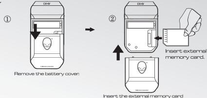
Insert the external memory can and replace the battery cover:
